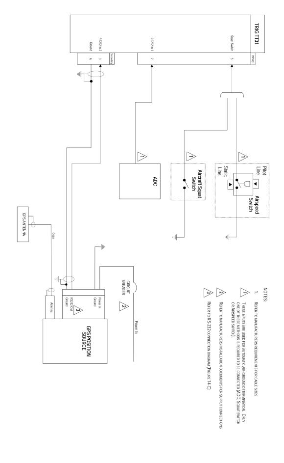
Figure 14-B Typical TT31 ADS-B Out Interconnect
