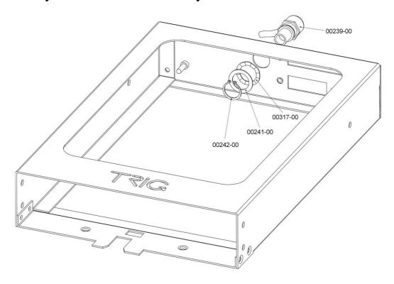
When the BNC is prepared, feed it through the TT31 mounting tray and attach the washer combination in the following order:
